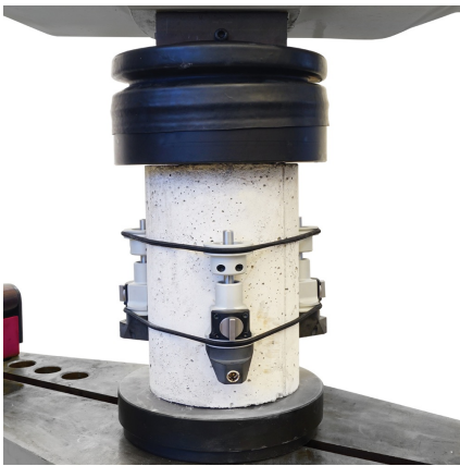
Elastic modulus test on concrete
